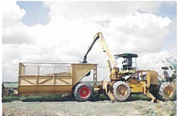
Bell Loader for more efficient gathering of cut canes at most Estates
