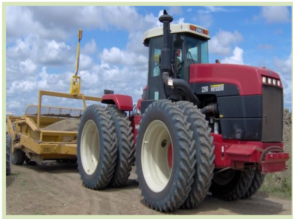
Buhler Versatile 290HP Tractors equipped with laser-levelling equipment
